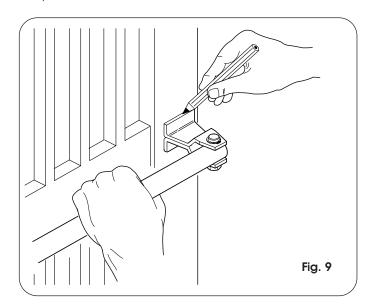
Spot weld the front bracket on the leaf, protecting the rod against any welding splatter.
