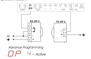
NOTE: If present remove the jumper from Pin 11
