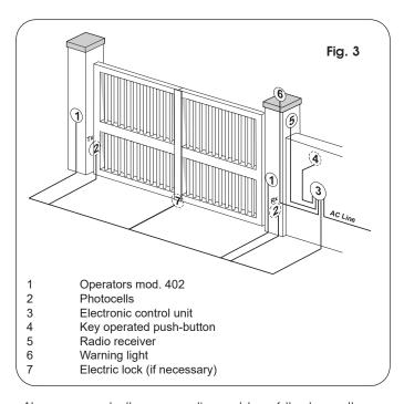
Always separate the connection cables of the low voltage accessories from the high voltage power cables. Use separate conduits to avoid interference.
