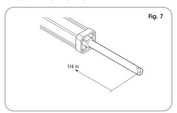
Push the front pin through the front mounting bracket then the piston rod to temporarily attach them together.
