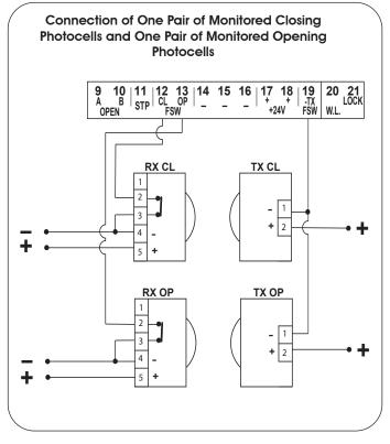
If an additional monitored opening safety device is needed it can be connected to the STP input. The "OP" parameter in the board configuration must be set to active
