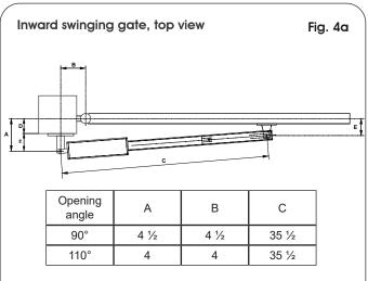
D: If greater that 2 in. a recess must be constructed
